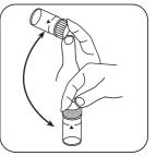
Dissolve tablet(s) by inverting.
