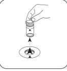
Remove the vial from the sample chamber.
