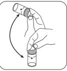
Dissolve tablet(s) by inverting.
