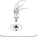
Remove the vial from the sample chamber.
